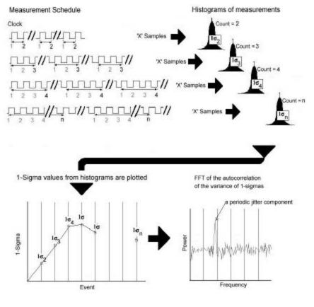
**Figure 6** The High Frequency Modulation Analysis increments the Stop Counters to build many histograms and plot the accumulation of jitter.
