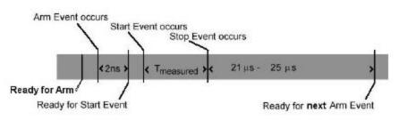
Figure 4 Measurement timeline when using External Arm
