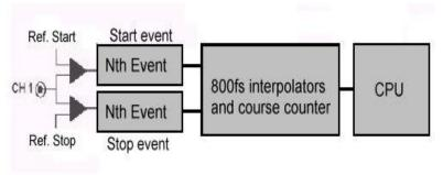
Figure 2 DTS simplified block diagram
