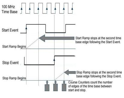
Figure 3 Diagram of time measurement.
