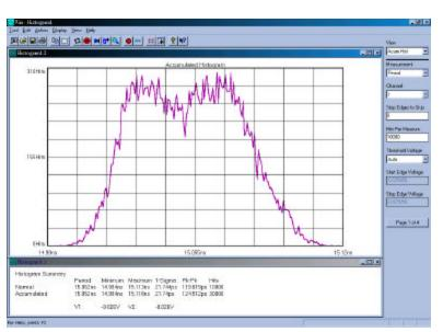
Figure 5 Shows a Histogram of period measurements
